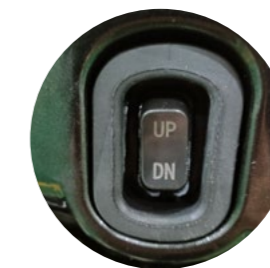
Power Tilt&Trim Switch
